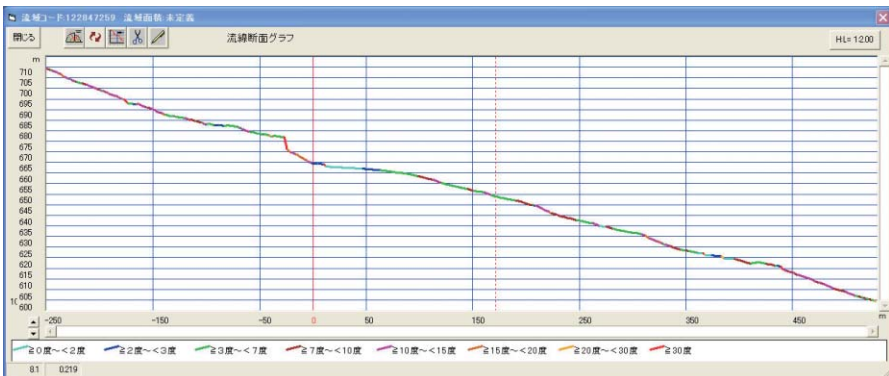
Fig-3 A longitudinal profile of a watercourse
