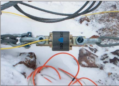
Abb4: Messzelle zur Seilkraftmessung Fig4: measuring cell for cable force measurement
