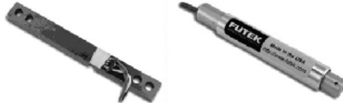
Fig6: The load cells used in the experiments to measure the force against the retarding elements. On the left, the non-protected model; on the right, the protected model.
