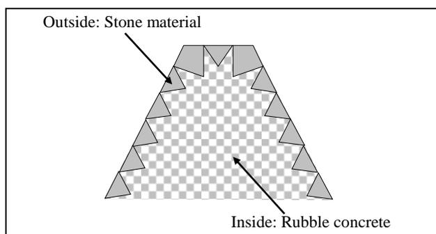
Fig. 7 Check dam with rubble concrete structure
