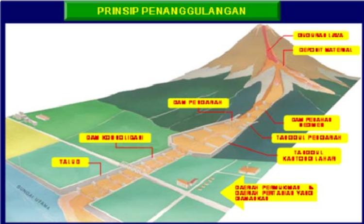
**Fig. 4** Debris flow disaster countermeasure model in a volcanic area (source: Mt. Merapi Volcanic Debris Control Project, Yogyakarta.)
