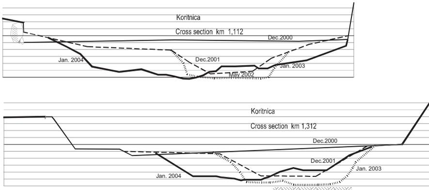
**Fig. 7:** The evolution of two cross sections of the Koritnica River after the debris flow event in November 2000. Vertical step is 1 m.
