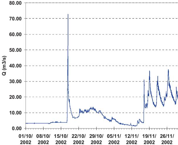
**Fig. 6:** Flood waves in October and November 2002, measured at the water level recorder in Kal-Koritnica.
