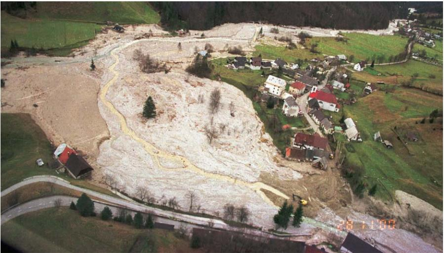
**Fig. 2:** Debris flow deposits in Log pod Mangartom (photo: November 28, 2000). The Predelica Torrent comes from the right and flows to the Koritnica River, coming from the left.
