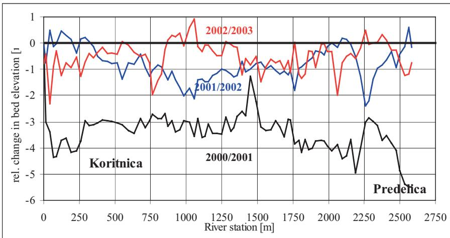
**Fig. 9:** Measured changes of the riverbed elevations of the Predelica Torrent and the Koritnica River in the area of Log pod Mangartom after the debris flow event in November 2000.
