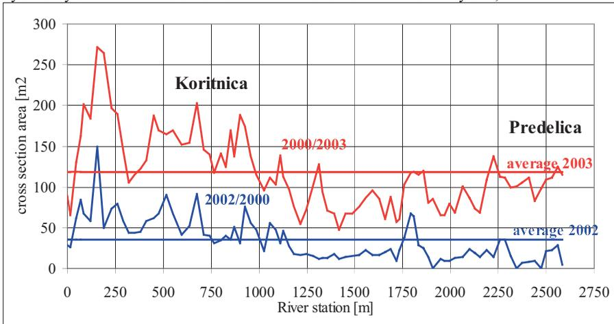
**Fig. 8:** Measured changes of the cross section areas of the Predelica Torrent and the Koritnica River in the area of Log pod Mangartom after the debris flow event in November 2000.
