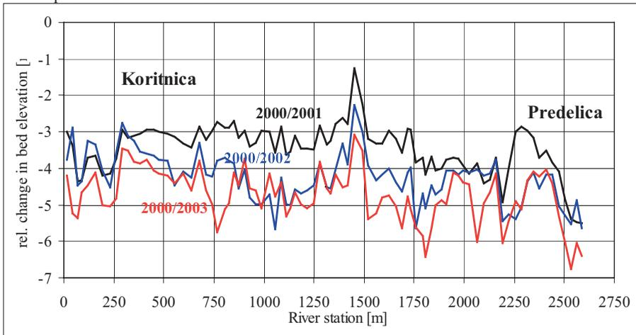
**Fig. 10:** Measured changes of the riverbed elevations of the Predelica Torrent and the Koritnica River in the area of Log pod Mangartom after the debris flow event in November 2000.
